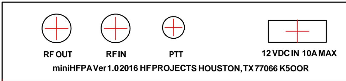
**Rear View: RF Connections, Control and DC Power Input**
